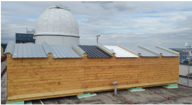
Figure 4 Experimental box with six roof samples in the first test run on the roof of CTU in Prague
