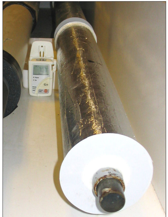
Figure 3. Samples in the horizontal environmental chamber
