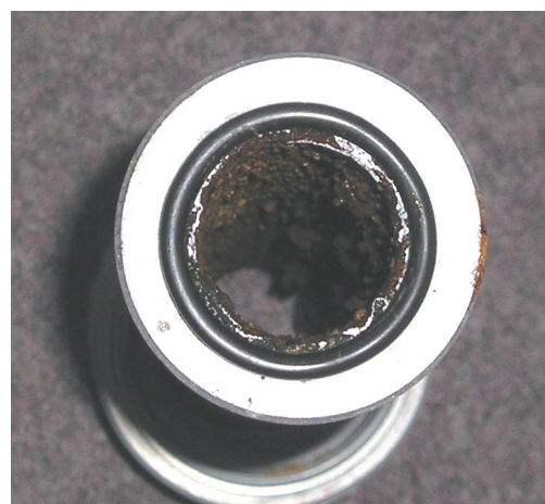
Fig. 7 Replacement inspection pipe (internal surface check) and EKOMAG tangential separator
